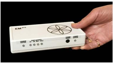
On the EM272, there are 5 lights on the left. The first one is the Charge status, (Green when fully charged; amber/red when low charge). The second and third lights show that the Nasal Probes (L and R) are attached. They glow green when in use. Lights four and five show that the Magnetic Discs (L & R) are attached. They also glow green when in use. On the Right is the Power button-
